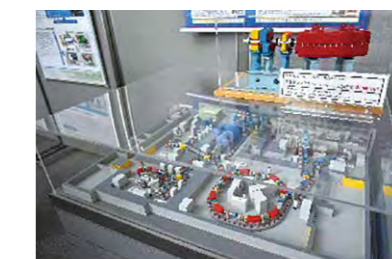
The combination of a microwave ion source ion implantation device, a tandem accelerator, and a synchrotron enables versatile applications in various research fields.
